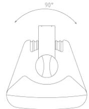
Once the bracket is fitted, support the speaker in position and attach top and bottom using the supplied screw caps and adjust to the required angle. Further mounting points are available at the rear of the speaker, should it be preferred to use different mounting methods (e.g. 129.130 – 129.124UK)
