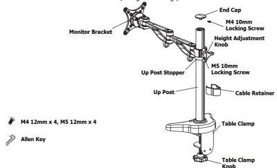
For this installation you will also require a tape measure and a Philips (cross) screw driver.
