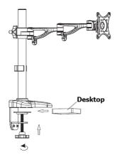
**Step 3** – Mounting screen. After checking the desktop mount is installed firmly, the monitor can now be installed on to the mount. Check the weight of the monitor is no more than 8kg before installing. Use the correct sized screws for your screen from the screws supplied and fit the screen on as shown in the diagram below. Tuck all cables into the cable management hook at the bottom of the bracket to finish the installation.
