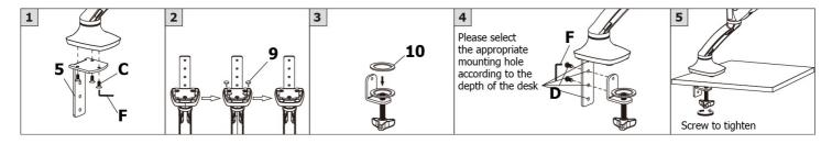
Option 2 – Assemble and mount via grommet
