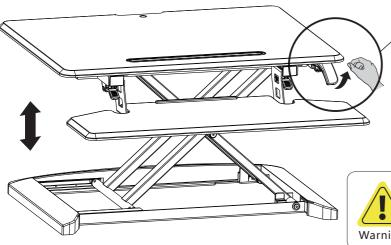
To adjust to the desired height take a firm grip on the worktop and press the adjustment lever on the right hand side. Take care when adjusting with a lighter load as it will adjust up quickly and could cause damage to your equipment or personal injury
