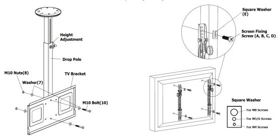
**Step 3** – Hook the TV bracket on to the drop pole and tighten the locking screw. Loosen the hand knob on the side of the drop pole for height adjustment, tighten to fix the position. The bracket can be tilted 0° to 12° and will pan 360°.
