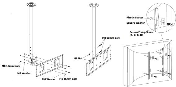
**Step 3** – Hook the TV bracket on to the drop pole and tighten the locking screw. Loosen the hand knob on the side of the drop pole for height adjustment, tighten to fix the position. The bracket can be tilted -5° to 15° and will pan 360°.
