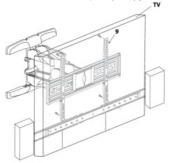
Alternatively, this bracket can be used as a low profile speaker wall mount to hide behind a TV set.
