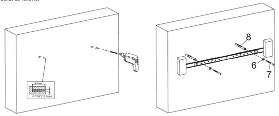
For plaster wall installation first of all find out where the wood stud is behind the wall using a stud finder. Then work out the height of the installation and ensure it is level using a spirit level. Use a pencil to mark where the mounting holes will be and use an electric drill to drill a hole that is around 4.5mm in diameter and 60mm deep. Install the wall bracket as follows.
