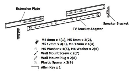
Step 1 - Assemble the bracket as shown below.
