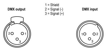
Connect the DMX output of the first unit in a DMX chain with the DMX input of the next unit in the chain. Always connect the the output of one unit with the input of the next unit unit all units are connected.
