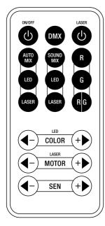
ON/OFF button – turn the unit on or off DMX button – set the unit to DMX mode Laser ON/OFF button – turn the lasers on or off
