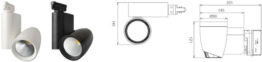
Fluxia TLF25 track lights are designed to be fitted into Fluxia single circuit, 2-wire 'H' track. With the circuit switched off, a lever at one end of the connection base can be switched across to retract the contacts, allowing the TLF25 to be inserted into the track.
