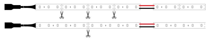
Each 5m reel of single colour LED tape is fitted with a 2.1mm DC jack socket for power input for easy connection to a power supply. This connector may be removed and stripped for bare wire connection if a 2.1mm jack is not fitted to the power supply.
