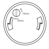
Each PIR has individual time adjustment on the rear of the sensor. To access this, rotate the front of the PIR a few degrees anti-clockwise against its rear cover and pull apart.
