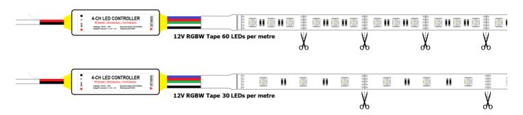
Each 5m reel of RGBW LED tape is fitted with a 5-pin connector for power input from an RGBW controller. Ensure that the V+, R, G, B and W pins are connected the correct way round.
