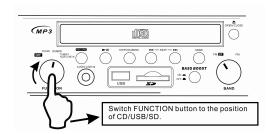
3. Press this button on the unit for 2 seconds to select the CARD-USB mode as below diagram:
