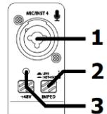
2. IMPED switch Press this button in to set the input impedance to instrument level or leave the button in the up position for a line level input. (instrument level is usually for pickups, such as those on a guitar. Electronic keyboards usually produce a line level output)
