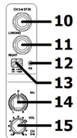
13. Level Sets the line input level to  $-10\text{dB}$  if pressed in or  $+4\text{dB}$  if not pressed in.
