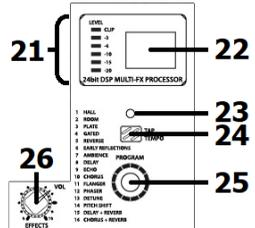
Press the encoder to confirm the selection, the display will stop flashing & selected program will be active.
