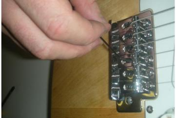
Once the desired action is achieved, all that remains is to set the vibrato tension and intonation. After tuning up all the strings, the spring claw may need tightening (or slackening) in the rear cavity to make the vibrato system "float" (note: some players prefer that the bridge lies completely flat against the body).
