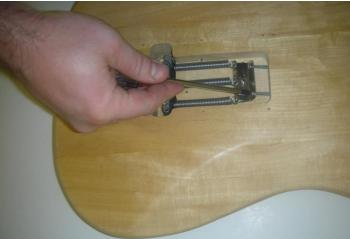
Lie the body face-up on a soft surface. Take the vibrato bridge and sit it into the routed section toward the rear of the body, allowing the sustain block (the metal block underneath the bridge) to hang into the hole through the body.
