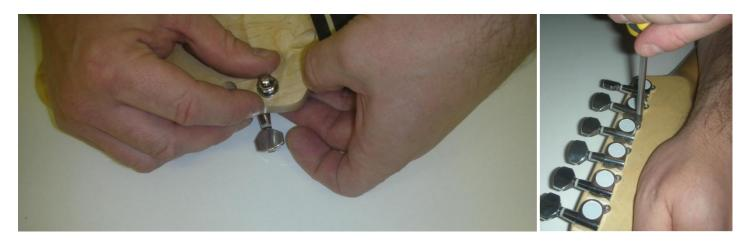
Before attaching the neck to the body, fit the tuning machine-heads to the headstock by inserting the thread through the pre-drilled holes and setting a washer and bush over it.
