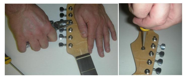
Fix the retaining screw through the loop on the rear of the gear housing into the pilot hole to hold the tuner in position. Then tighten the nut on the front face of the tuner until firm using a spanner
