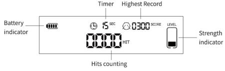
Set the time by short pressing the MODE button, and the record for that time is displayed next to the drum symbol. Countdown will begin on the first strike of the pad and stop when timed out, showing your score.
