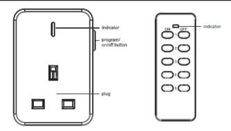
**Un-programming a socket** from a remote is also possible by unplugging the socket from the mains. Press and hold the program/on/off button on the side of the socket while plugging it back in, keep the button pressed for around 5 seconds until the LED indicator begins to flash. Finally release the button to finish the reset and the LED indicator should stop flashing.
