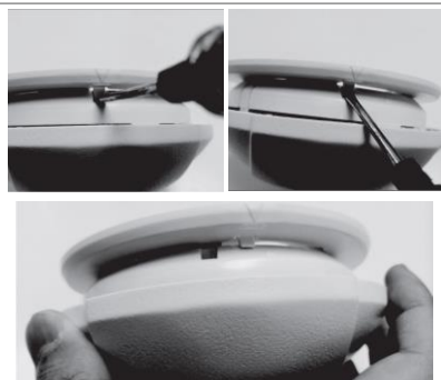
Figure 6 – Push Back the snap lock and turn the Alarm anti-clockwise
