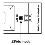
Alternatively, the L25U can be powered by an external 12Vdc source (such as car battery) connected via a 2.1mm DC jack located between the pistol grip and rear cover hinge (a lead is supplied for connection to a car cigar lighter socket).
