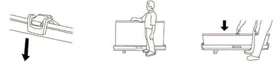
• After the screen is fully retracted into the case, close the lid and secure both clasps on the case. Finally, tuck the stabilizing feet under the case. The case is ready to store away
