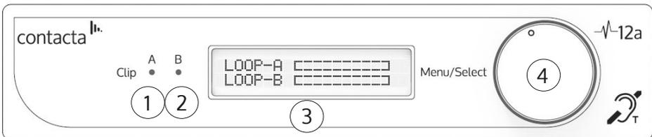
1. **Clip Status Light** - When lit, this status LED indicates the signal on Hearing Loop A is clipping (see Troubleshooting on page 23 for appropriate solutions).
