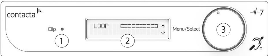
1. **Clip Status Light** - When lit, this status LED indicates the signal on the hearing loop output is clipping (see Troubleshooting on page 23 for appropriate solutions).
