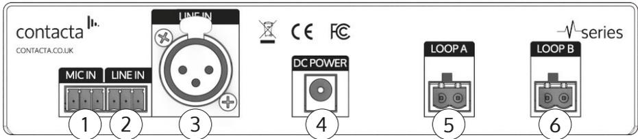
1. **Microphone Input** - 3.81mm Euro-block balanced microphone input (12V phantom power via 680 $\Omega$ ).
