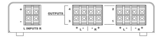
• The terminals on the rear of the speaker selector will accommodate up to 14-gauge cable which will suffice for long connections (greater than 100 Feet of wire). For shorter distances, 16 or 18-gauge wire will suffice. For behind the wall installations, we recommend using UL Class 3 approved cable (marked "CL3") for compliance with local building regulations.
