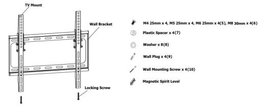
For this installation you will also require a pencil, tape measure, electric drill, stud finder and a Philips (cross) screw driver.
