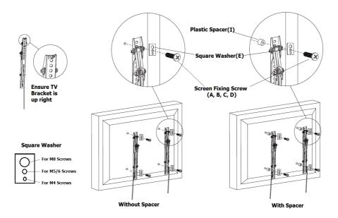
**Step 3** – Hook the TV bracket on to the wall mount and gently rest the TV against the wall as shown below. Use a screw driver to fix the locking screw in until the TV is completely fixed to the bracket.
