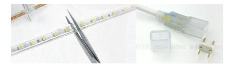
The end of the powered strip will need to be fitted with an end cap (Pack of 10 = 153.853UK), using silicone glue to secure it. This will also reinstate the waterproof protection to the strip. Fitting shrink-tubing can add additional weatherproofing and protection.
