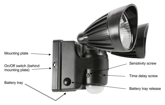
A robust battery powered floodlight with PIR that provides a bright twin LED beam when triggered in the hours of darkness. It's easy to fit bracket and battery operation makes it a quick and simple addition to any property where security is needed. The twin 3W COB LED's give off an impressive 400 lumens and the PIR sensor operates at up to 10m distance at 120° coverage angle.
