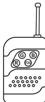
Press to activate, release to stop fog output.
