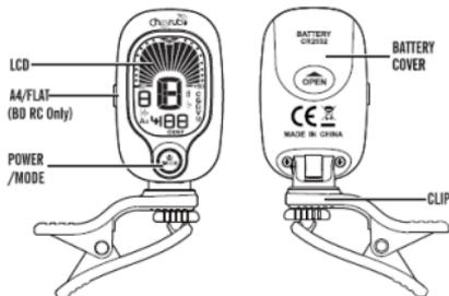
When the battery charge is low, the LCD will become dim. Please replace the battery as soon as possible.
