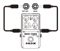
You can connect external pedals, using send & return jack, to enrich the effect sound of NUX Stageman. Signal forwarding to external pedals from Send Jack already been processed by built-in equalizer but not built-in effects.
