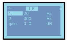
In the menu for the HF or LF crossover settings, there is a field for 1, 2, and gain. "1" is the lowest frequency, "2" is the highest frequency and "gain" can be used to adjust the level of signal to that frequency range, which can be used to boost or cut overall treble or bass response.
