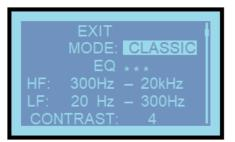
Turning to "MODE" and pressing the selector offers 5 x DSP profile settings: NORMAL, JAZZ, POP, CLASSIC and CUSTOM. Rotate the selector to the required profile and press to select.
