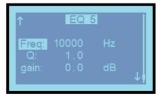
Scrolling down the settings using the rotary selector will highlight "Freq:" for setting the centre frequency of the selected EQ band. Press the selector to adjust the frequency in Hertz (Hz). Press the selector again to save the setting.
