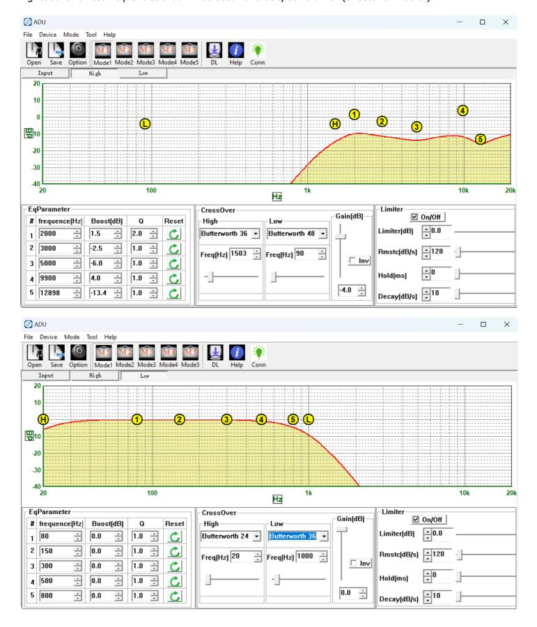
The EQ nodes are editable in the **EqParameter** section in the same way as for the main Input tab. These nodes can be clicked and moved around the screen or adjusted numerically by frequency, Boost and Q settings at the bottom left of the window. Either click on the  $\checkmark$  buttons or enter the value directly. Clicking "Reset" returns all values to default settings.
