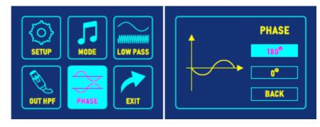
calculate which phase will be most effective, but often it is best to try both settings and choose which is most effective for a strong sub output. This can be further fine-tuned using the DELAY function.
