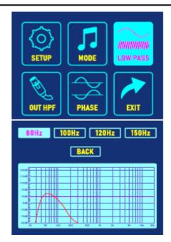
When the required cutoff frequency is set, turn the encoder to highlight BACK and press to return to the main menu.
