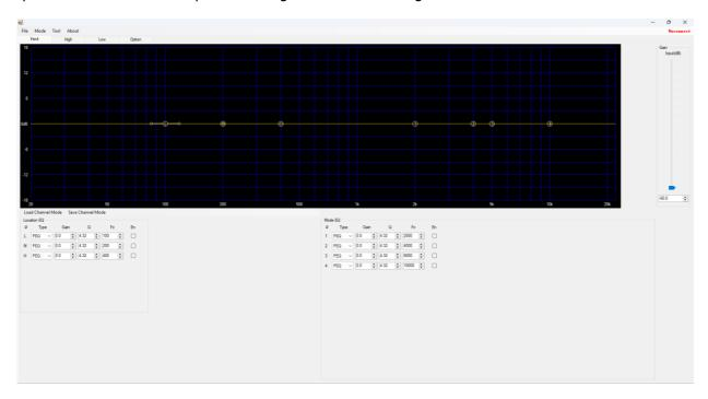
Double click on the red Unconnect label at the top right side of the window and a pop up will appear showing the detected serial port and baud rate. Click "OK" and the label on the top right side will show Connected. (if this fails, check alternative serial port options in the drop down menu and/or re-start the PC or software)
