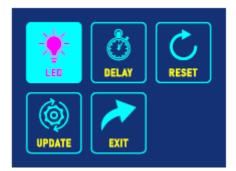
In the menu, rotate the encoder to highlight DELAY and press to set it ON or OFF and to set the delay time in milliseconds (ms)
