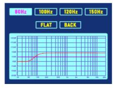
When the required HPF cutoff preference is set, turn the encoder to highlight BACK and press to return to the main menu.
