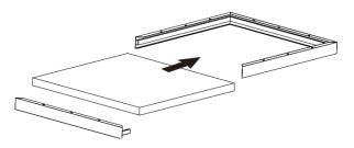
Push the lamp forward and connect it to the power supply, then install the fourth side.
