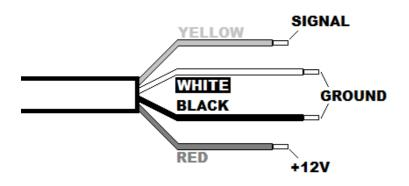
The amplifier can be operated from any 12Vdc power supply capable of delivering up to 1.2A current. It is recommended to use a filtered, noise-free power supply to avoid hum or whistling noises in the audio (e.g. item ref 660.451UK)
