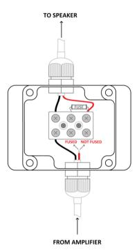
For ceiling speakers, the ceramic terminal block is located on the rear (upper) side of the speaker basket. Again, connect the input via the thermal fuse if one is fitted.
