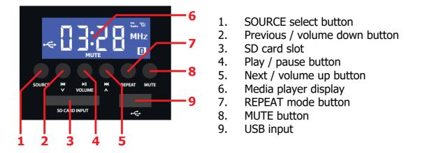
RM60B, RM120B, RM240SB and RM360SB mixer-amplifiers are fitted with a built-in media player. This section comprises a Bluetooth receiver, USB/SD audio player and FM tuner. Pressing the SOURCE select button (1) will step through "bt" (Bluetooth), USB, SD card and FM tuner modes.
